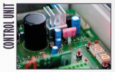
Easy to access due to its positioning in the upper part of the body- this enables the total and precise management of the barrier by the digital control unit.
